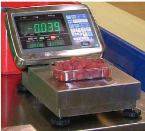
***The MCI Solution was to supply the 'Shortie' version of its acclaimed AJA DP Traffic Light Checkscale, with WiFi built in. This is networked with the MCI Myrias Pack Weight Optimising Software with a unique Operator feature. The DP scale displays by number exactly + or- individual fruit need to be added or taken away from the punnet. An error free system. At the same time Myrias in the background runs Average weight optimising correcting scale tolerances in real time to minimise give away***
